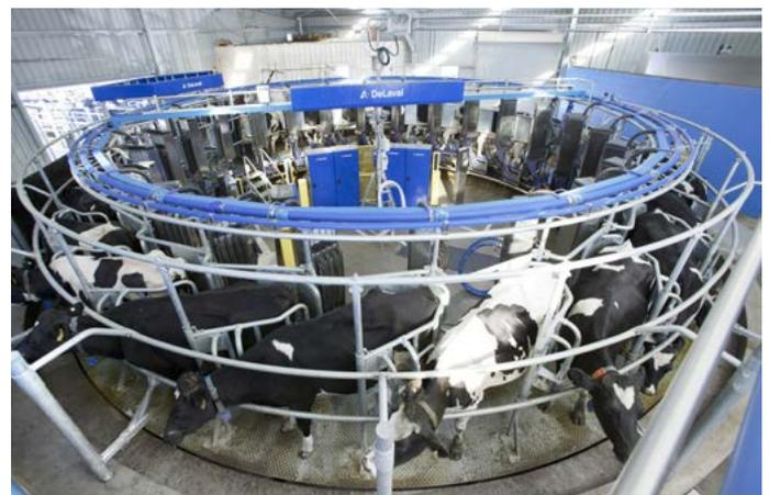
The robotic rotary is a 24-bail internal herringbone rotary. Cows stand at a 30-degree angle with their heads facing out and their rumps facing in. The 30-degree angle enables the five centrally located robots to approach the cows from the side (between the front and back leg). Two robots are dedicated to teat preparation, two to cup attachment and the fifth robot disinfects teats after milking. The robotic rotary can milk about 90 cows an hour.
