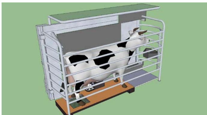
throughput (8-10 cows per hour) than the robotic rotary. There are two styles of multi-box units available; which has a single robot servicing two parallel boxes (the robotic arm sits in between the two boxes); and another which has a single robot servicing up to five boxes in series (end to end).
