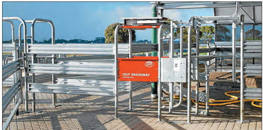
The Lely Grazeway is a set of smart gates that directs cows to either fresh pasture breaks or the feedpad, depending on how the gates have been programmed.
